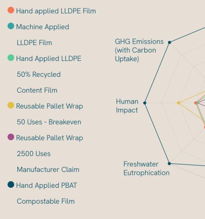
Figure 3: Spider Web Chart Overview of LCA Impacts for Stretch Films and Alternatives
