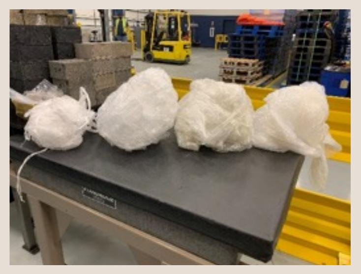
Figure 3: Machine-applied shrink film uses half of the material than a hand-applied alternative (from left to right: Control machine-applied, control hand-applied, PCR, compostable)
