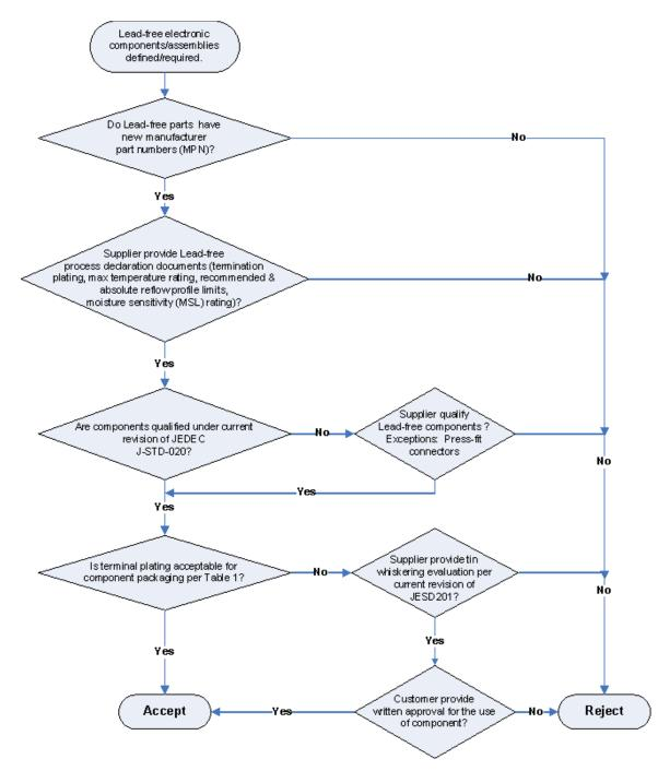
Figure.1: Flex' procurement flow diagram for Lead-free electronic component
